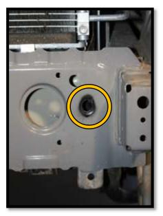
• Apply the Tightening bracket on the inside of the chassis mount behind the opening enlarged to 12 mm.
